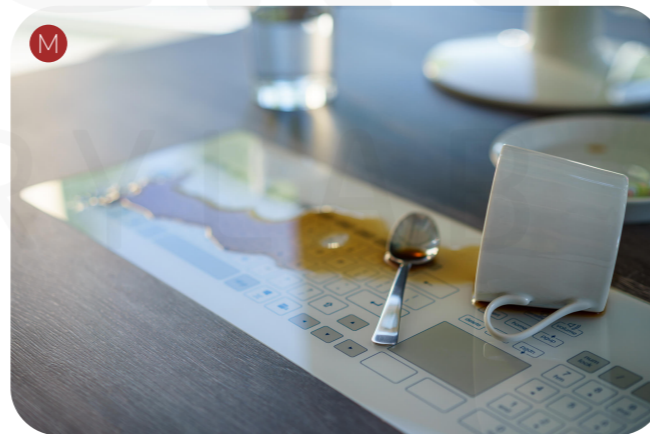
TEST-PLACE-KEYBOARD-GLASS-RECESSED Embedded capacitive keyboard with integrated touchpad and number block Operating surface made of glass IP65 Can be washed and disinfected, so complies with high hygiene standards Special buttons for locking keys, sensitivity and volume USB-Type: USB-A, cable length 2,1 m USB-Compliance: USB 2.0 compliant Supported operating systems: Win®, MacOS® & Linux® 482 x 179 mm, touchpad 60 x 42 mm
